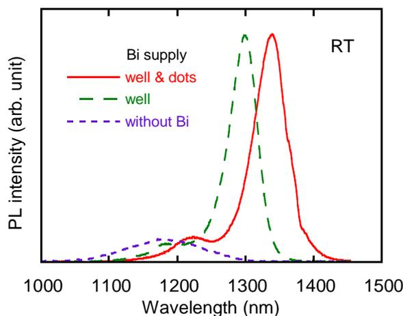
**Figure 3.** PL spectra for three In(Ga)As-QD samples: grown without Bi (dotted curve), grown with Bi supply only for the well layer growth (broken curve), and grown with Bi supply for both of the well layer and QD growth (solid curve).
