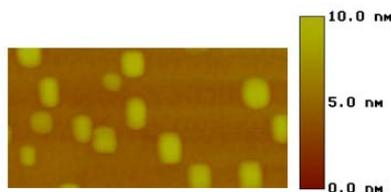
**Figure 7.** AFM image ( $0.25 \times 0.5 \mu\text{m}^2$  area) of an In(Ga)As-QD sample covered with thin InGaAs layers, for which Bi was supplied during the growth interruption. Growth interruption time was 12 seconds.
