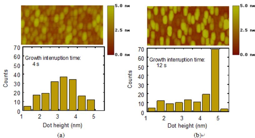
**Figure 6.** AFM images ( $0.25 \times 0.5 \mu\text{m}^2$  area) and corresponding dot-height histograms ( $0.5 \times 0.5 \mu\text{m}^2$  area) of the In(Ga)As QDs covered with thin InGaAs layers: growth-interruption times were 4 seconds (a), and 12 seconds (b). Bi supply was stopped during the growth interruption.
