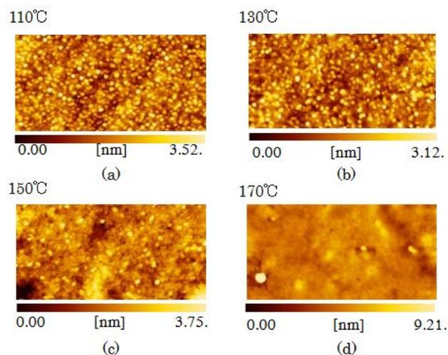
**Figure 12.** AFM images of the samples, for which Bi and Ge layers were deposited in the temperature range from 110 to 170°C. Bi and Ge thicknesses were fixed at 0.5 and 1.2 nm, respectively. AFM scanning areas were 0.5 x 1.0 μm<sup>2</sup>.
