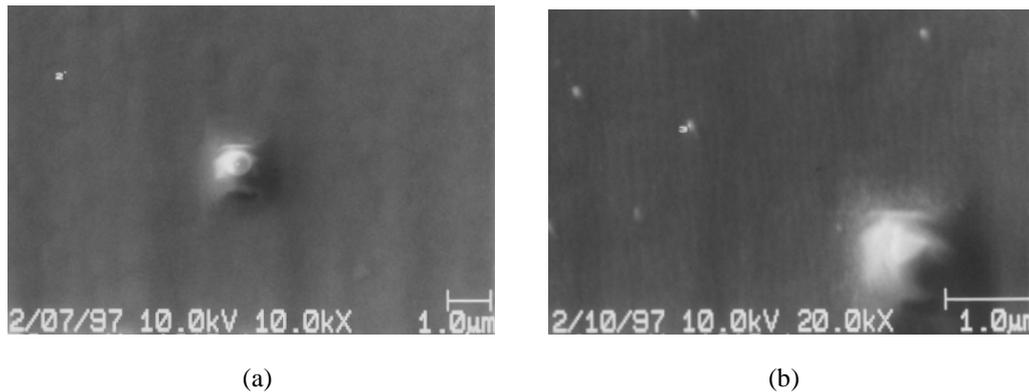
**Figure 1.** SEM images of an InGaAs layer grown on an InP substrate for AES analysis: Initial surface of the InGaAs covered with thin InP layer (with a hillock) (a), and the surface after Ar-ion spattering (small particles are unexpectedly appeared) (b). Small numerical characters ("2" and "3") appeared in these pictures are markers for AES analysis. This sample was grown for our previous study on Bi-containing alloy. Bi was supplied during the InGaAs-layer growth.
