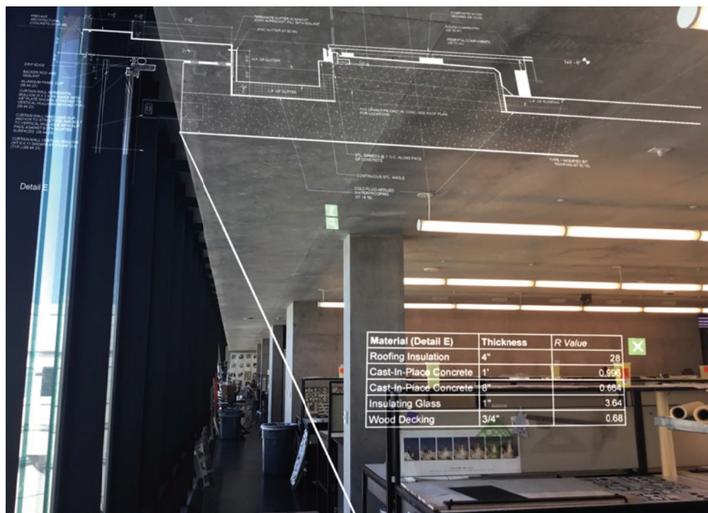
Figure 8. In-situ roof detail with table of R-values
