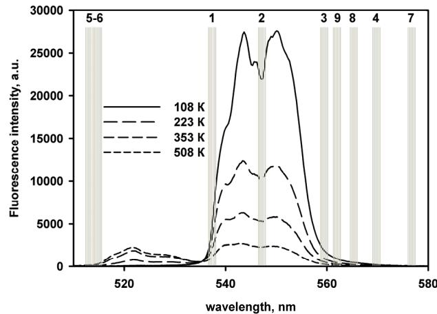
**Figure 3.** Fluorescence spectra of Er-doped glass considered and spectral intervals, for which the temperature prediction by the scmwiPLS method is characterized by a minimum value of RMSEP<sub>min</sub>. The numbers above the intervals show the order of their selection in the model.
