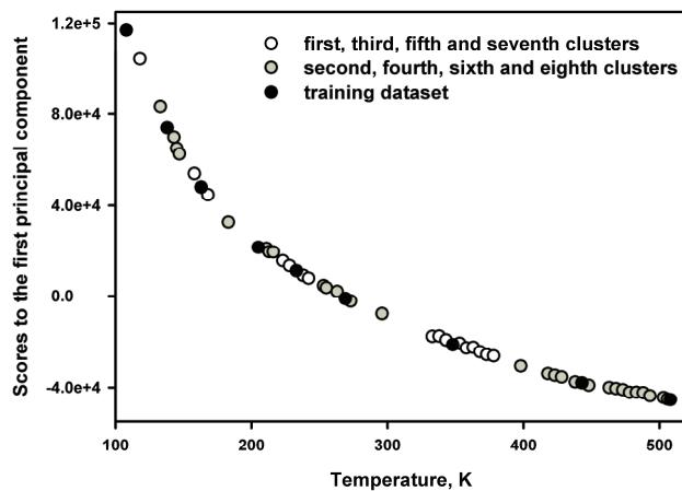
**Figure 1.** Dependence of scores to the first principal component on temperature for fluorescence spectra of a 0.5 mol% ErF<sub>3</sub> doped glass of 98MgCaSrBaYAlF<sub>14</sub>-2Ba(PO<sub>3</sub>)<sub>2</sub>, which was used to perform a hierarchical cluster analysis to determine the training dataset for temperature calibration by the PLS method.
