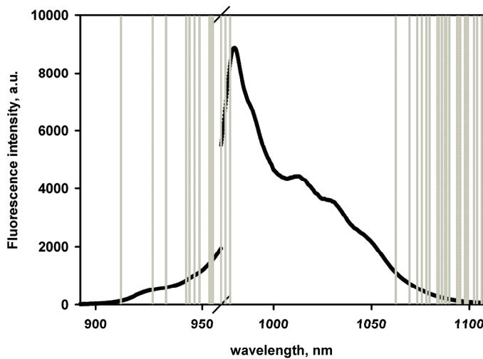
**Figure 4.** Fluorescence spectrum of a Yb<sup>3+</sup>:CaF<sub>2</sub> at the temperature of 339 K and spectral intervals, for which the temperature prediction by the scmwiPLS method is characterized by a minimum value of RMSEP.
