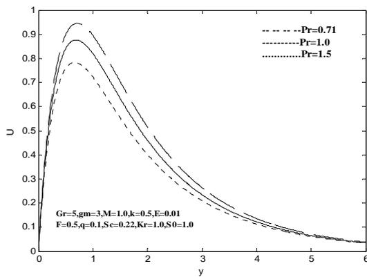
Fig 5(a). Velocity profiles for various values of  $Pr$ .
