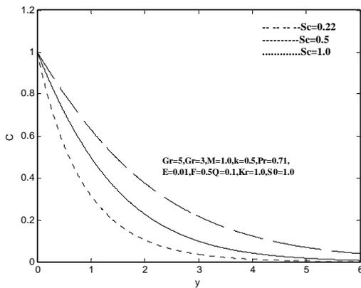
Fig 10. Concentration profiles for various values of  $Sc$ .
