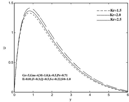
Fig 9. Velocity profiles for various values of  $Kr$ .
