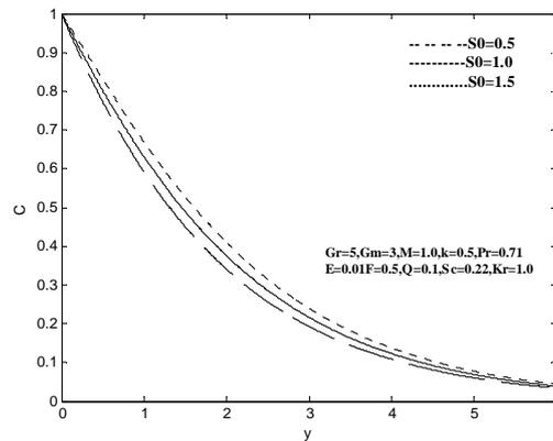
**Fig 12.** Concentration profiles for various values of  $So$ .
