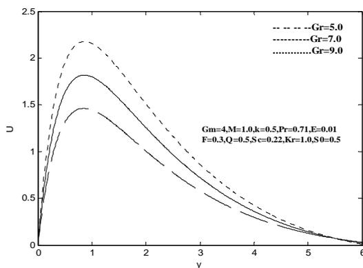
Fig 1. Velocity profiles for various values of  $Gr$ .
