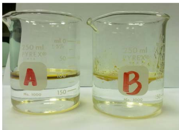
Figure 1. Digital images of (A) motor oil emulsion, (B) motor oil emulsion mixed with hydrophobic nano silica.
