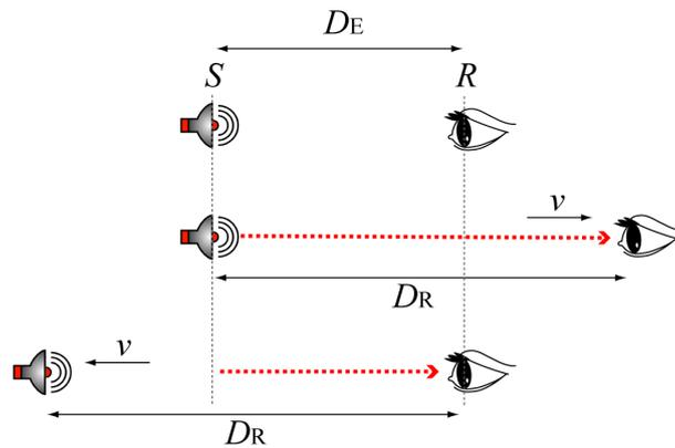
**Figure 1.** A light pulse is emitted by a source ( $S$ ) when spaced from a receiver ( $R$ ) by  $D_E$ . Just like a ball thrown between two players, light travels through a static medium relatively to which either  $S$  (middle line) or  $R$  (bottom line), is considered immobile.
