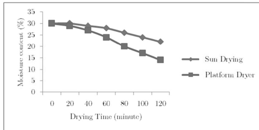
**Figure 4.** Relationship between moisture content and drying time of the paddy rice dried using platform and sun drying methods
